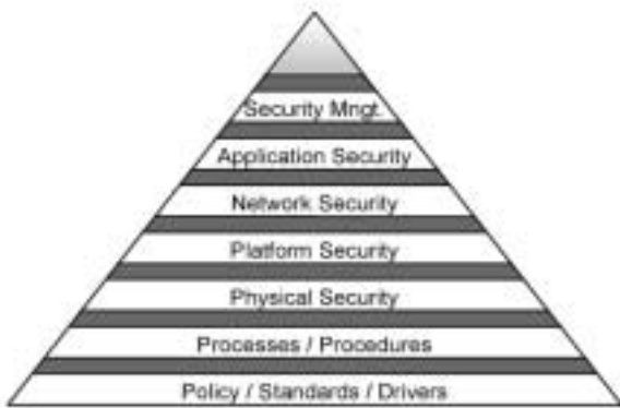
Figure 1. The internal security design of each node. This figure differs from the standard one because each level provides unique interface based on metadata. Dark levels represent metadata levels, which will be used as access points for probes.
